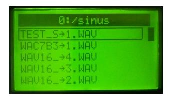
To play a WAV file on the output of the device, simply select the desired file with the rotary knob and press "OK - rotary knob".
