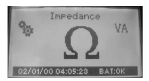
Connect the "+" and "-" terminals of the tester to the line to be measured (the polarity does not matter). Press the rotary knob or the "ON" key and select the desired measurement frequency using the rotary knob. Either:
