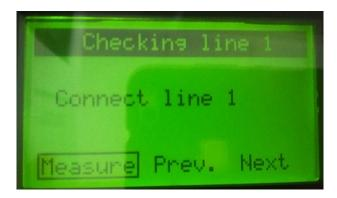
The "Prev." and "Next" buttons can be used to increment or decrement the number of the line to be tested.
