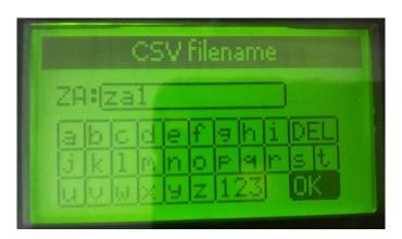
A filename can be entered using the virtual keyboard. Up to 12 characters are permitted. The characters are selected using the rotary knob and validated by pressing it (OK - rotary knob). It is a good idea to name the file with the name of the zone to be tested.
