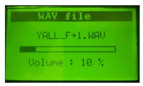
During playback, a bar indicates the state of progress. The output volume level can be adjusted with the rotary knob.
