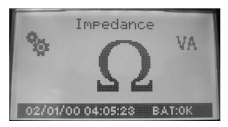
After connecting the "+" and "-" terminals of the tester to the line to be measured, press the knob to start measuring. The measurement is taken at a frequency of 1000Hz.
