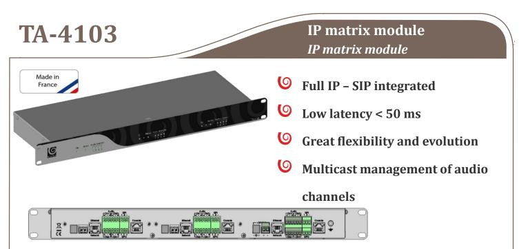
The matrix module **TA-4103** (rack-mounting unit) enables to get a public address system through IP network. Twelve configurable flows (input and/or output) can be managed. It is also featured with 6 GPI and 6 GPO. The **TA-4103** is a converter of analog lines into digital lines. It guarantees transmission of audio signal without compression distortion.
