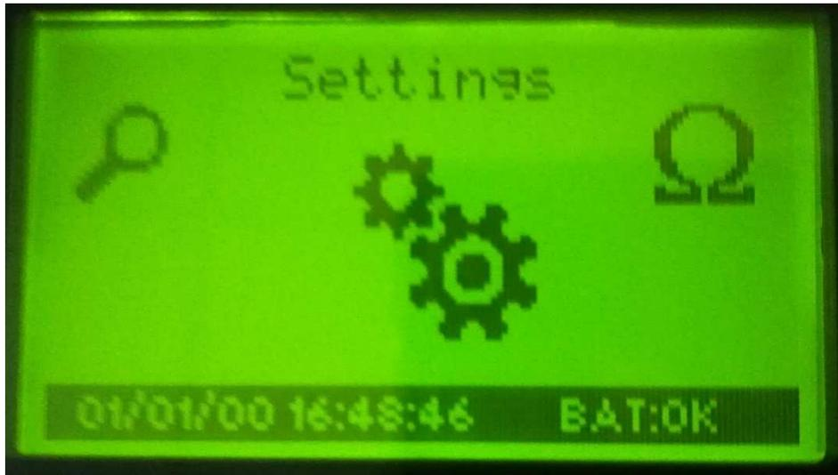
Press the rotary knob or the "Enter" button to access to the following menu.
