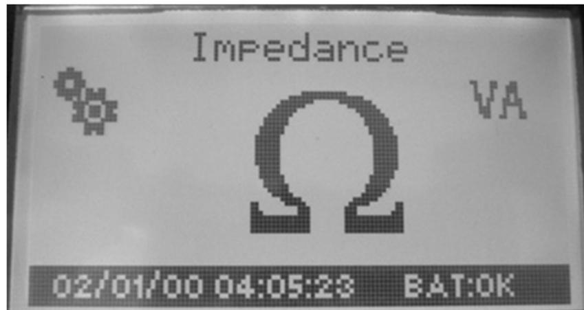
After connecting the "+" and "-" terminals of the tester to the line to be measured, press the knob to start measuring. The measurement is taken at a frequency of 1000Hz.
