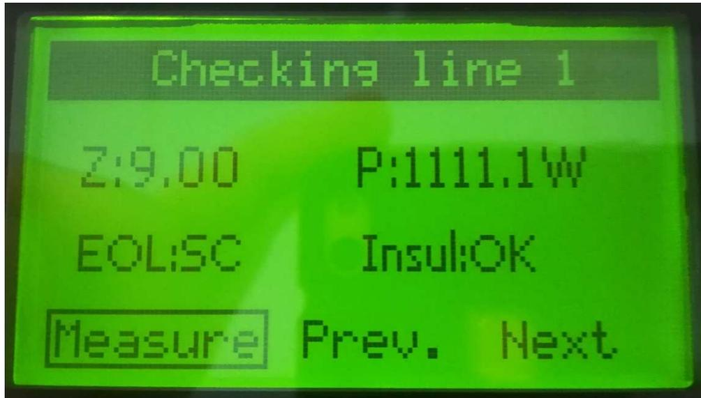
These results are automatically recorded in the file that was named previously in the "LOGS" directory at the root of the SD card.
