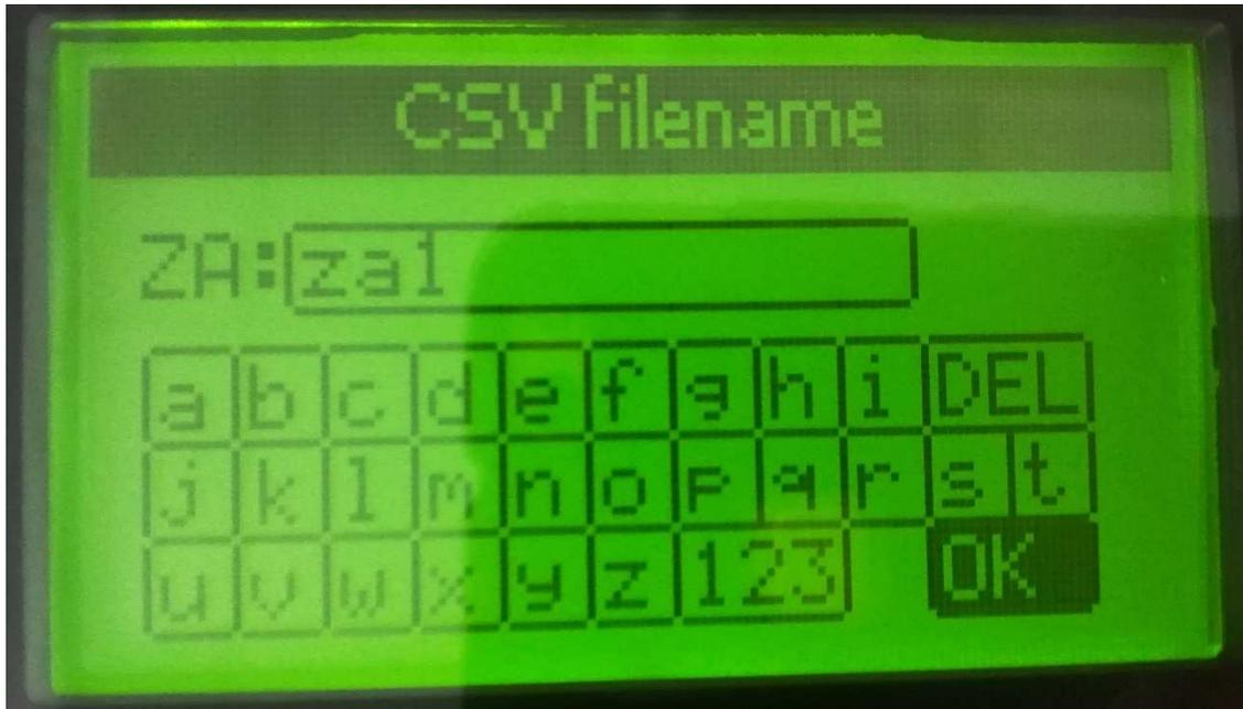
A filename can be entered using the virtual keyboard. Up to 12 characters are permitted. The characters are selected using the rotary knob and validated by pressing it (OK - rotary knob). It is a good idea to name the file with the name of the zone to be tested.
