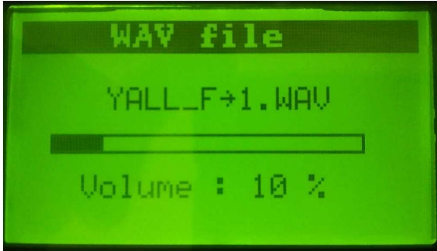
During playback, a bar indicates the state of progress. The output volume level can be adjusted with the rotary knob.
