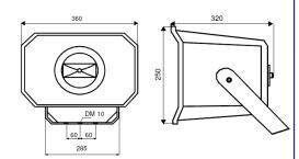
Its body out of ABS, its stainless steel screws and fork out of aluminium are perfect for harsh environments and guarantee an enduring installation.
