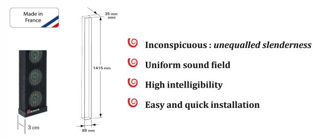
The **RC-3020** is a column-type sound speaker fitted with 5-cm low speakers distributed in « LINE ARRAY » architecture. It guarantees a uniform sound field for sitting as well as standing listeners, and optimizes pressure level decay, according to distance, 4dB(A) up to 6dB(A): gain of 9dB(A) at 13m compared with a traditional speaker.
