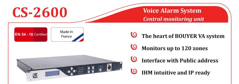
The **CS-2600** is the centralizing part of BOUYER voice alarm system. It is equipped with an emergency interface for emergency microphone on front panel and with a digital message player. Provided with LCD display on front panel, it is easily configured and consulted.
